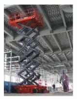
Working Height 5.8m to 18.2m Load Bearing 227kg to 680kg Gradeability 25%, 30%, 40%
